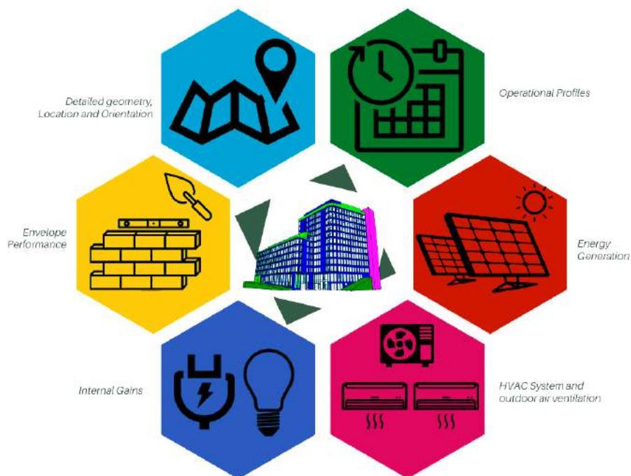
Figure 21: Inputs to a building energy model [121]
